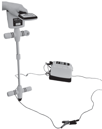
Configuration for Testing the Conductive Attachment
