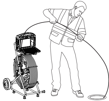
Improper placement and pushing may result in kinking the pushrod
