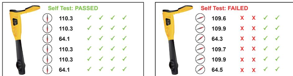
If the unit fails the test, try again in a more interference free area. If it continues to fail, return the unit to Vivax-Metrotech or one of its approved repair centers for investigation and repair.
